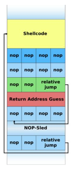
Illustration of a NOP-sled payload on the stack.
