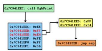
An instruction from ntdll.dll to call the DbgPrint() routine contains the i386 machine opcode for jmp esp.
