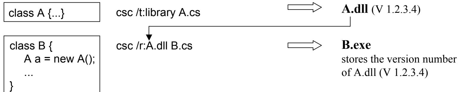
***Version number is checked when the assembly is loaded***
