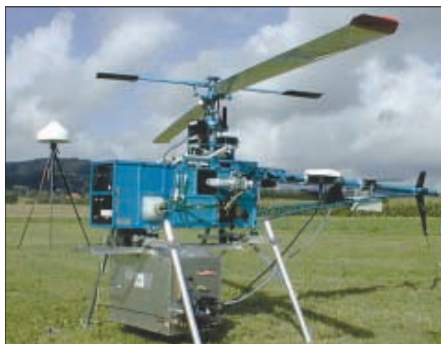
Figure 3. The model helicopter and the OLGA control system (aluminum box).
