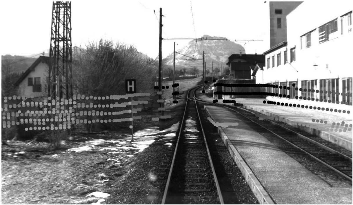
Figure 4-7: Display of laser echoes within the video picture
