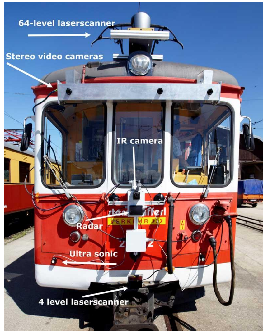
Figure 4-2: Sensor installation on the prototype autoBAHN vehicle
